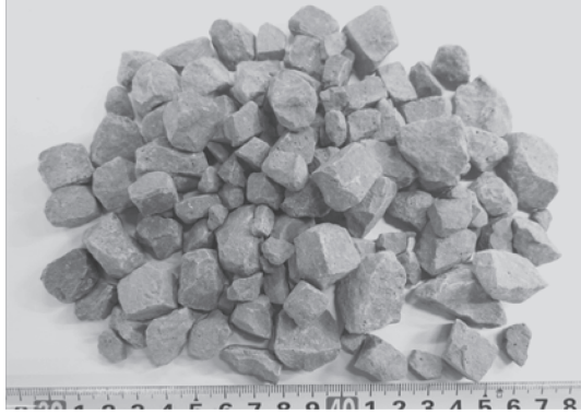
写真 5 低吸水率高炉スラグ粗骨材 Photo 5 BFG with low water absorption
